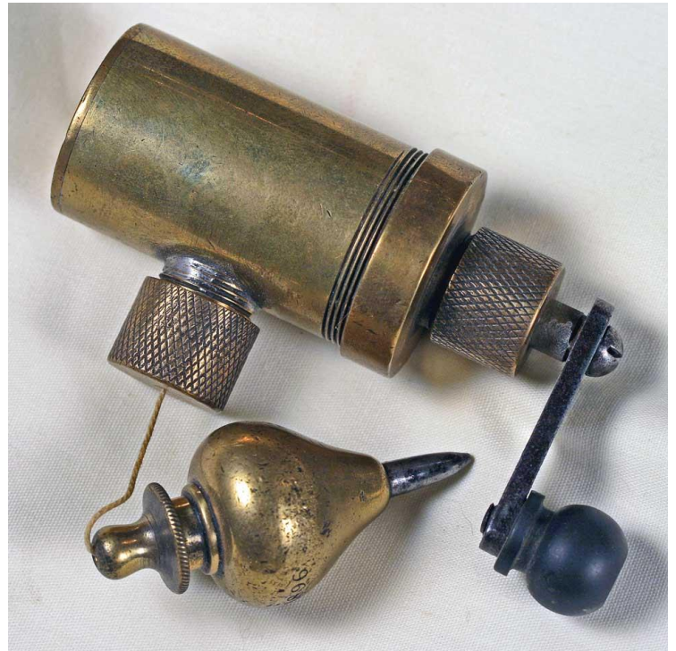
ND #456 SMETHWICKS PATENT 1896, ENCLOSED CRANK REEL W/ SMALL TURNIP BOB. MANUFACTURERS MARK APPEARS ON END OF REEL CASING. DATE 1896 ALSO APPEARS ON TURNIP PLUMB BOB. SMETHWICK PATENT, LONDON, 1896
