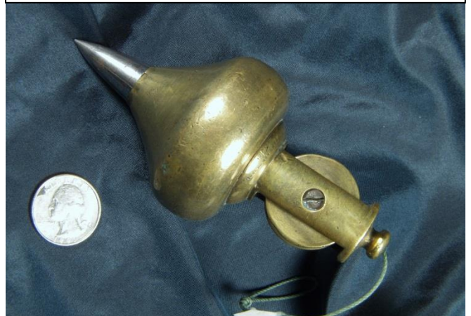
RARE STANLEY TRAUT PATENT, PAT'D APRIL 28, 1874 REEL IN NECK , PROTOTYPE SHAPE, NOT IN PRODUCTION ND# 665
