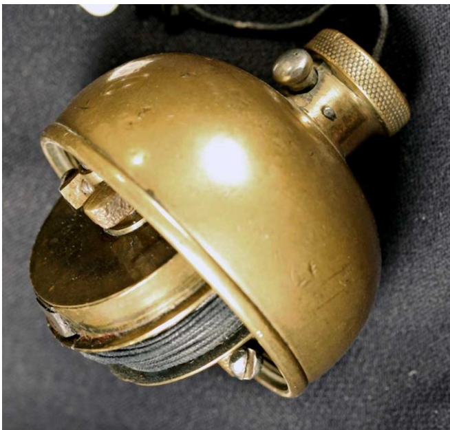
ND # 463 CLOCKWORKS MECHANISM, "LALLIE" WITH BRAKE; 4.5 x 1.6 in 10.1 oz FINE, LIGHT USE, MECHANISM WORKS
