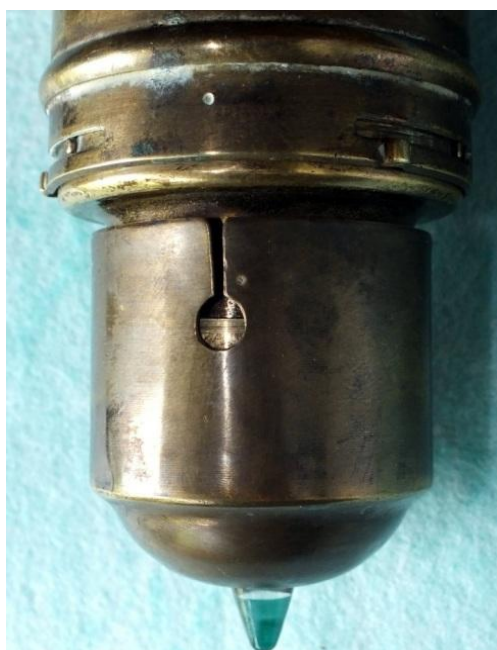
This brass diaphragm covers the lens and lets only free the lighted colored tip as sighting device
