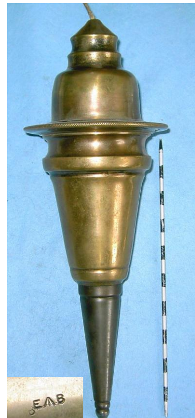
The largest English bridge builders plumb bob from my collection. 11 in, 8+ lbs (28 cm 3,7 kg)
